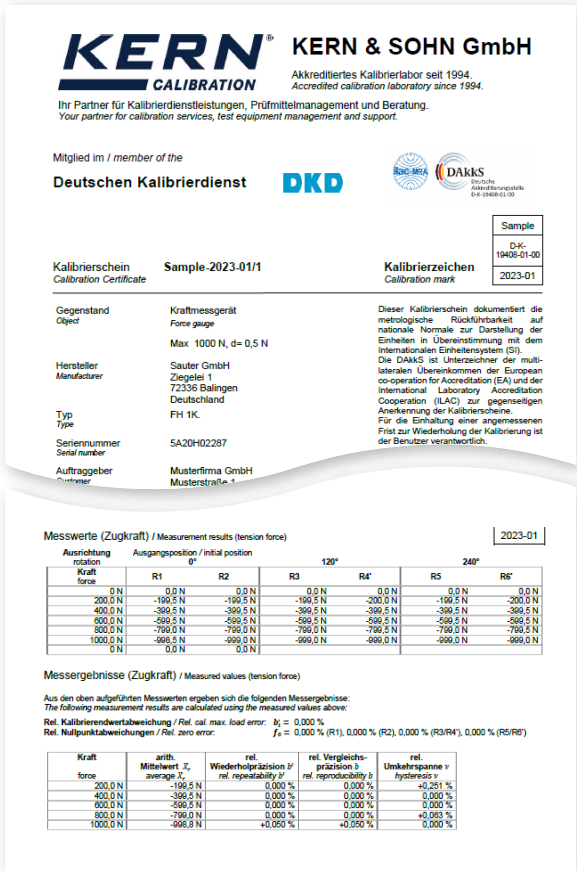
Calibration certificate with accreditation symbol for force gauges (extract)
